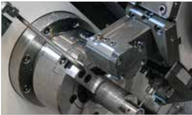
Chuck Air Blow (Upper Chuck)
